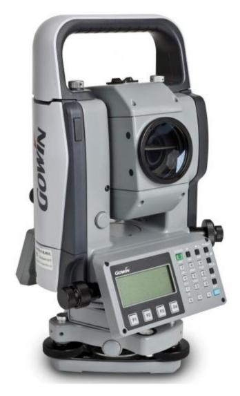
The new Gowin TKS-202N serie Power by TOPCON total station combines the traditional Gowin rugged field-ready quality and accuracy with economical, compact design that is perfect for everyday measuring and positioning applications such as topo and construction layout.
